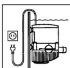
**For your own safety we recommend that you make a drip loop with the power cord. This drip loop prevents any water running along the cord from reaching the electrical socket.**
