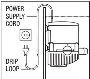
The “drip loop” is that part of the cord below the level of the receptacle, to prevent water travelling along the cord and coming in contact with the receptacle.
